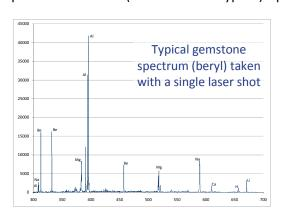
throughout the spectrum. The figure at left illustrates a portion of a single-shot LIBS spectrum of a gemstone. Major and minor elements can be resolved, and the 14,000+ points in a typical spectrum can be expanded to reveal lines separated by less than 0.5 nm in the UV range. Overall, the broadband spectrometer used in the Insight™ allows excellent sensitivity to low light levels at an affordable price point.
